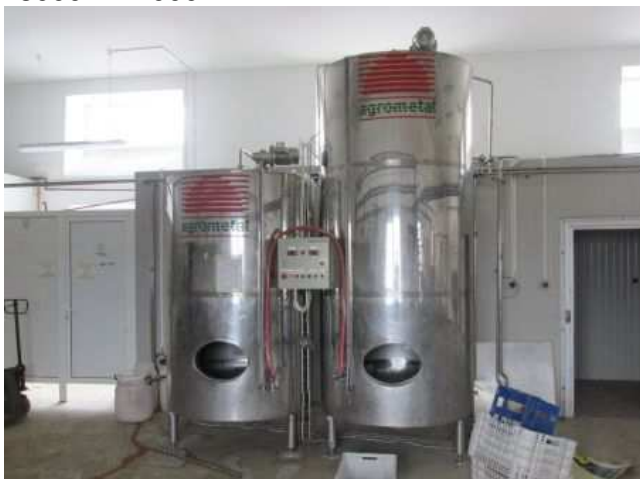
Ad 6 Pasterizator mlijeka P5-2 (2000 L/H)
