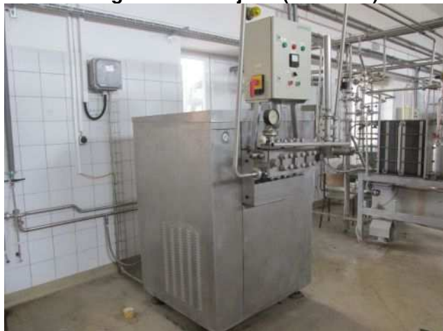
Ad 7 Homogenizator mlijeka (2000 L/H)
