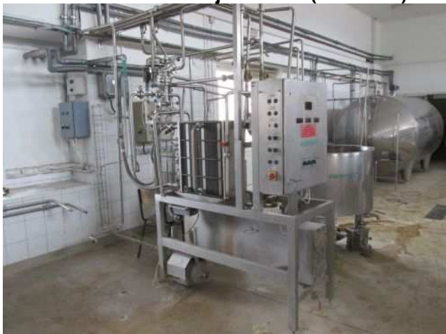
Ad 6 Pasterizator mlijeka P5-2 (2000 L/H)
